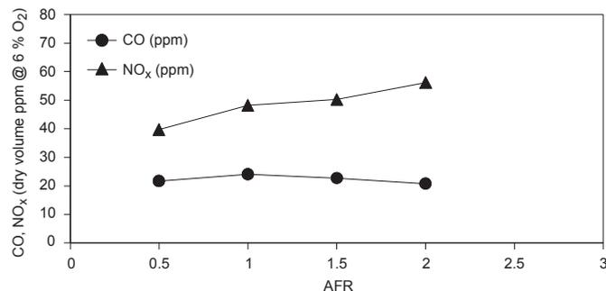
Fig. 7. Effect of AFR on CO and NO<sub>x</sub> emissions for diesel.
