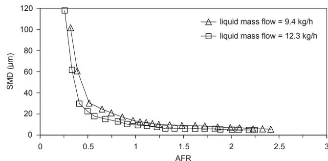
**Fig. 5.** SMD as a function of AFR for two water mass flow rates.
