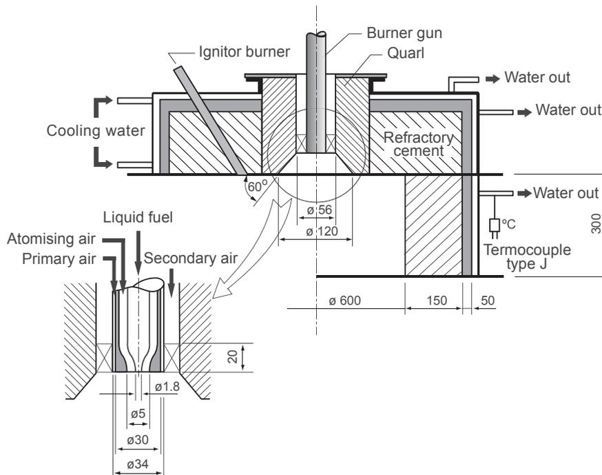
Fig. 2. Schematic of the furnace roof and burner arrangement.
