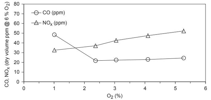
Fig. 9. Effect of excess air level on CO and NO<sub>x</sub> emissions for biodiesel.
