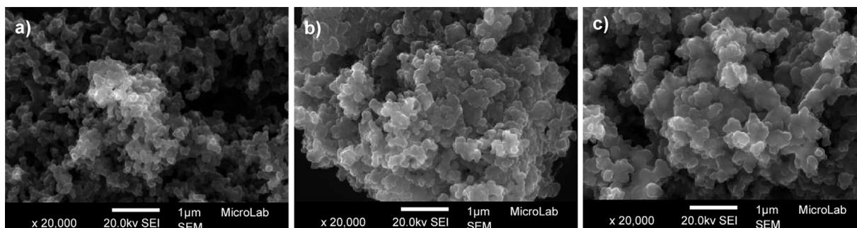
Fig. 11. Typical SEM images of PM. a) Biodiesel, AFR = 0.5, flue gas  $O_2$  = 2%; b) biodiesel, AFR = 2, flue gas  $O_2$  = 2%; c) diesel, AFR = 2, Flue gas  $O_2$  = 2%.
