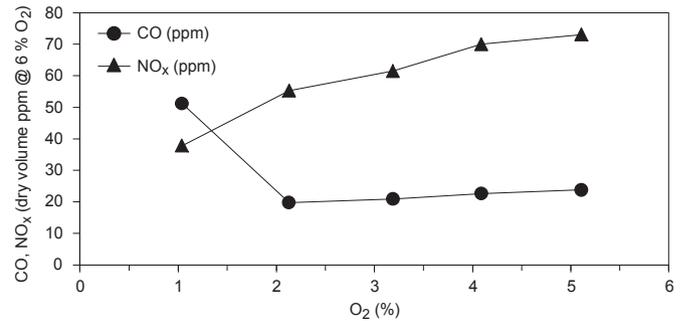
Fig. 10. Effect of excess air level on CO and NO<sub>x</sub> emissions for diesel.
