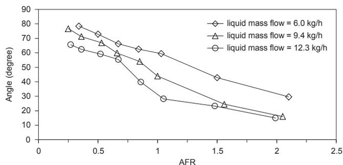
**Fig. 4.** Spray cone angle as a function of AFR for three water mass flow rates.
