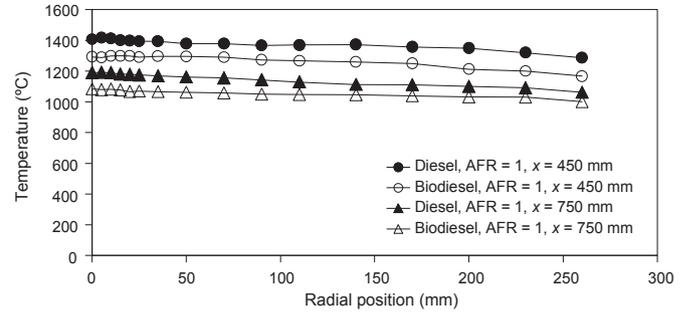
Fig. 8. In-flame temperature radial profiles for biodiesel and diesel firing. (x represents the axial distance from furnace roof).
