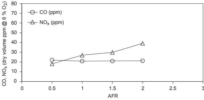
Fig. 6. Effect of AFR on CO and NO<sub>x</sub> emissions for biodiesel.
